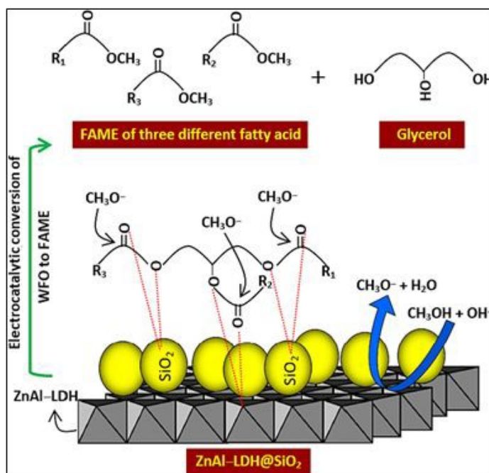
Figure 10: Suggested mechanism of transesterification process using ZnAl/LDH-SiO 2 composite.
