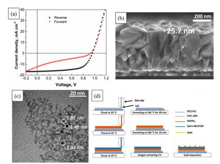
Fig. 13 (a) J-V curves of a device based on SnO<sub>2</sub> QDs. (b) FESEM image showing the cross-section of the SnO<sub>2</sub> layer. (c) TEM image of the SnO<sub>2</sub> QD. (d) Schematic of the device fabrication process. Reproduced with permission. <sup>193</sup> Copyright 2022, MDPI
