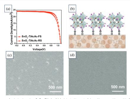
Fig. 14 (a) Typical J-V curves of a device based on  $SnO_2$ -TiAcAc. (b) Anticipated impact of depositing perovskite on thin films of TiAcAc-doped  $SnO_2$ nanoparticles. FESEM images of (c) SnO<sub>2</sub> layer deposited on FTO and (d) SnO<sub>2</sub>-TiAcAc deposited on FTO. Reproduced with permission. 194 Copyright 2021, Wiley.
