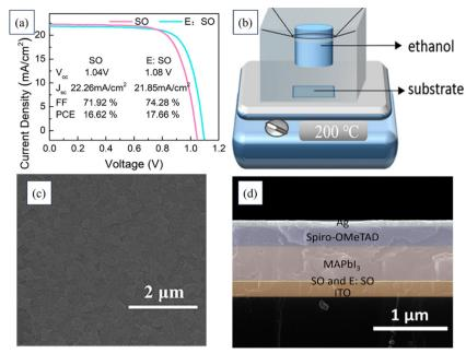
Fig. 23 (a) J-V curves of a device based on the SnO<sub>2</sub> film with and without ethanol vapour treatment. (b) Schematics of the ethanol vapour experimental set-up. SEM images of (c) SnO<sub>2</sub> layer deposited in ethanol vapour and (d) cross-section of the tested device. Reproduced with permission.<sup>202</sup> Copyright 2020, Elsevier.
