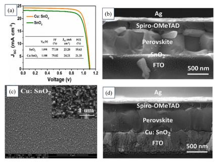
Fig. 18 (a) J-V characteristics of photovoltaic devices utilizing SnO<sub>2</sub> and a 5% copper-doped tin dioxide (Cu:SnO<sub>2</sub>) ETL. FESEM images of (b) crosssection of the device with SnO<sub>2</sub> as the ETL, (c) Cu-doped SnO<sub>2</sub>, (d) cross-section of the device with Cu-doped SnO<sub>2</sub> as the ETL. Reproduced with permission. 197 Copyright 2022, Elsevier.
