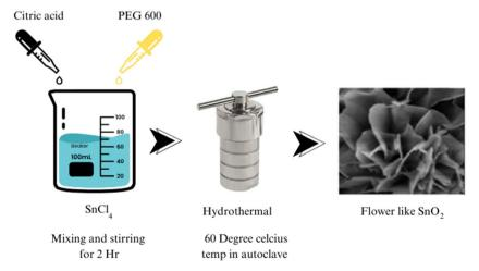
Fig. 2 Synthesis of a flower-like morphology of SnO<sub>2</sub> using the hydrothermal method.
