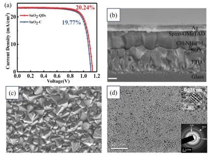
Fig. 12 (a) J-V characteristic curves from forward and reverse scans. (b) FESEM image of the cross-section of a tested device. (c) SEM image of SnO<sub>2</sub> coated on an FTO substrate. (d) TEM image of SnO<sub>2</sub>. Reproduced with permission. (e) TeM image of SnO<sub>2</sub> Reproduced with permission.
