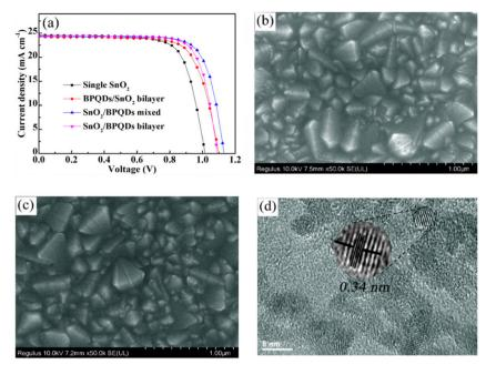
Fig. 15 (a) J-V curves of single SnO<sub>2</sub>, BPQDs/SnO<sub>2</sub> bilayer, SnO<sub>2</sub>/BPQDs mixed, and SnO<sub>2</sub>/BPQDs bilayer ETL-based PSCs, FESEM images of (b) single SnO<sub>2</sub>, (c) SnO<sub>2</sub>/BPQDs mixed sample. (d) TEM image. Reproduced with permission. <sup>154</sup> Copyright 2022, American Chemical Society.
