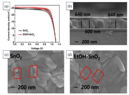
Fig. 20 (a) J-V curves of devices based on SnO<sub>2</sub> and EtOH-SnO<sub>2</sub> as ETLs. FESEM images of (b) cross-section of the device, (c) deposited SnO<sub>2</sub> layer, and (d) EtOH-SnO<sub>2</sub>. Reproduced with permission. <sup>199</sup> Copyright 2022, Elsevier.
