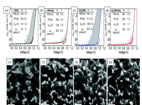
Fig. 21 Reverse (R) and forward (F) J-V scans and stabilized PCE (s-PCE) derived from MPP tracking of champion PSCs with (a) c-SnO<sub>2</sub>, (b) c-NP-SnO<sub>2</sub>, (c) c(Li)-SnO<sub>2</sub>, and (d) c(Li)-NP-SnO<sub>2</sub> ETLs. Top SEM images of perovskite thin films deposited on (e) c-SnO<sub>2</sub>, (f) c-NP-SnO<sub>2</sub>, (g) c(Li)-SnO<sub>2</sub>, and (h) c(Li)-NP-SnO<sub>2</sub> ETLs. Reproduced with permission.<sup>200</sup> Copyright 2022, Royal Society of Chemistry.
