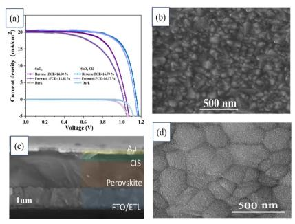
Fig. 19 (a) J-V curves of devices based on  $SnO_2$  and modified  $SnO_2$  as the ETL. FESEM images of (b)  $SnO_2-Cl_3$  sample coated on FTO, (c) cross-section of a device based on SnO<sub>2</sub>-Cl<sub>3</sub>, (d) perovskite deposited on the SnO<sub>2</sub>-Cl<sub>3</sub> ETL. Reproduced with permission. <sup>198</sup> Copyright 2022, Elsevier.
