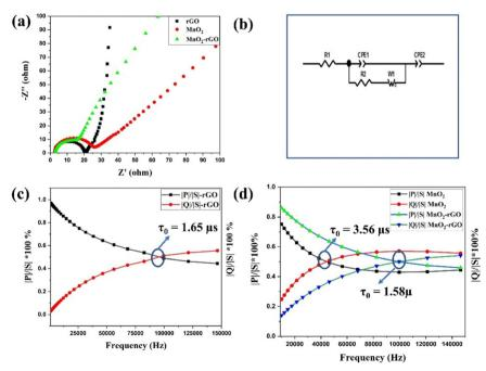
Fig. 7 (a) EIS spectra of rGO, MnO<sub>2</sub> and the MnO<sub>2</sub>-rGO electrode, (b) equivalent fitted circuit of the EIS data. Plot between |P|/|S| and |Q|/|S| along with frequency (Hz) for the (c) rGO-electrode and (d) MnO<sub>2</sub> and MnO<sub>2</sub>-rGO-electrode.
