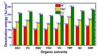
Fig. 3 Desolvation energy values of K<sup>+</sup>, Na<sup>+</sup>, and Li<sup>+</sup> in typical organic solvents. Abbreviations: dimethyl formamide (DMF), butylene carbonate (BC), trimethyl phosphate (TMP), vinylene carbonate (VC), fluoroethylene carbonate (FEC), ethyl methyl carbonate (EMC), propylene carbonate (PC), diethyl carbonate (DEC). The data was derived from ref. 35 and 36.
