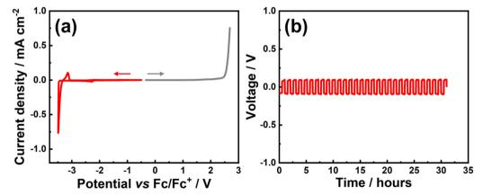
Fig. 28 Electrochemical stability of 0.5 M KTFSI in Pyr<sub>13</sub>TFSI ionic liquid at 298 K. (a) Cyclic and linear sweep voltammograms conducted at a scan rate of 1 mV s<sup>-1</sup> to assess the cathodic (in red) and anodic (in grey) limit. (b) Voltage profiles during galvanostatic deposition and dissolution of potassium in potassium symmetric cells performed at a current density of 6.4 μA cm<sup>-2</sup>. Figures adapted from ref. 5 with permission. Copyright 2019 Wiley-VCH.
