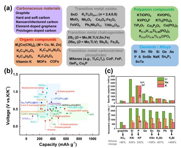
Fig. 25 (a) Exemplars of anode materials for potassium-ion batteries.<sup>297–305</sup> (b) Ragone plot showing the average voltages attained by selected anode materials along with their theoretical capacities. (c) Theoretical capacities of alloy-based anode materials compared to graphite in potassium-, sodiumand lithium-ion battery configurations, and (d) corresponding volumetric capacities. Figures adapted with permission.<sup>42</sup> Copyright 2020 American Chemical Society
