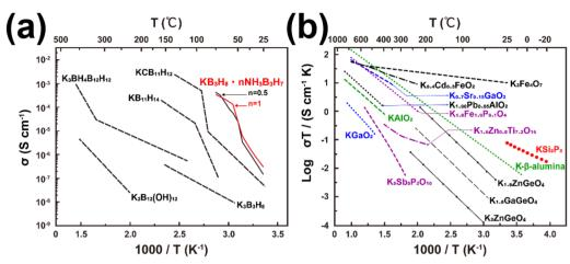
Fig. 32 Exemplars of inorganic compounds that can be utilised as solid-state potassium-ion conductors. (a) Borohydrides. 452 (b) Oxides (including cristoballite-type polyanion frameworks), antiperovskite phosphides and sulphides. Graph plotted from data derived from ref. 456-458, 460-472, 477 and 478. Figure (a) reproduced from ref. 425 with permission. Copyright 2022 American Chemical Society.
