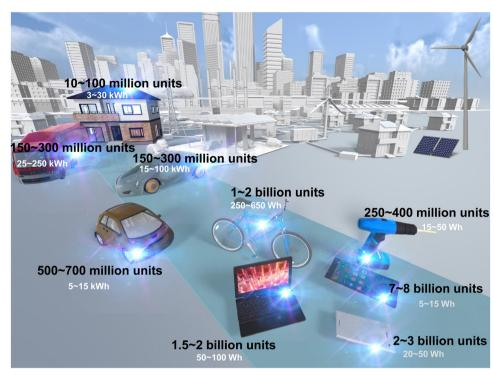
Fig. 1 Projected number of energy devices and battery size, including those for portable electronics and large-scale energy storage in electric vehicles. Rechargeable batteries, like the current LIB, are expected to be extensively utilised
