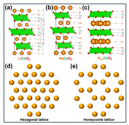
Fig. 18 Layered frameworks of (a) LiCoO<sub>2</sub>, (b) NaCoO<sub>2</sub> and (c) K<sub>0.5</sub>CoO<sub>2</sub>. (d) Arrangement of mobile cations in a hexagonal lattice as exemplified in LiCoO2 and NaCoO2. (e) Arrangement of mobile cations in a honeycomb lattice as exemplified in potassium-deficient K<sub>0.5</sub>CoO2.
