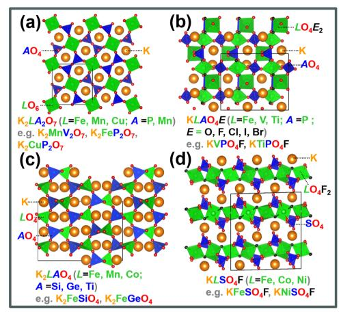
Fig. 12 Selected crystal structural frameworks of polyanion-based compounds. (a) Pyrophosphates and pyrovanadates, (b) KTiOPO<sub>4</sub> and derivative compounds, (c) cristoballite-type orthosilicates, orthogermanates and orthotitanates, and (d) fluorosulphates. Unit cells are highlighted in black boxes.
