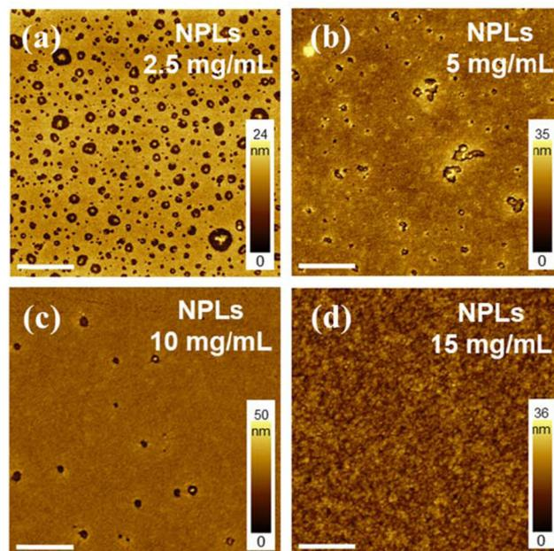
Fig. 3 AFM surface morphologies of the blade-coated composite films under fixed NPLs to P-TPD ratio (1 : 2), with NPL concentration of (a)  $2.5 \text{ mg mL}^{-1}$ , (b)  $5 \text{ mg mL}^{-1}$ , (c)  $10 \text{ mg mL}^{-1}$  and (d)  $15 \text{ mg mL}^{-1}$ . All white scale bars represent  $2 \mu\text{m}$ .
