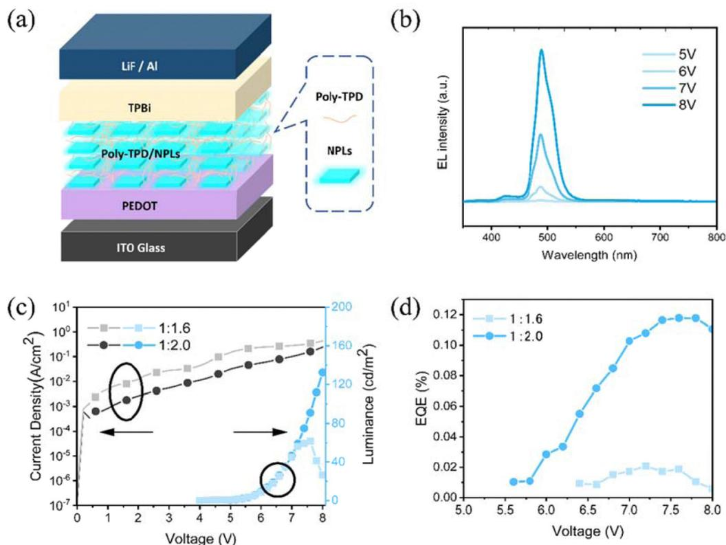
Fig. 7 (a) Device structure, (b) EL spectra of the optimized device with the active layer thickness 45 nm and prepared from a  $15 \text{ mg mL}^{-1}$  NPL suspension with a polymer mixing ratio of 1:2. (c) Current density–luminance–voltage curves and (d) EQE–V curves of sky-blue LED with different ratios of NPLs to P-TPD.
