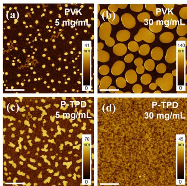
Fig. 2 AFM surface topography of the blade-coated films with different ratios of polymers at  $10 \text{ mg mL}^{-1}$  NPL concentration. (a) PVK at  $5 \text{ mg mL}^{-1}$ ; (b) PVK at  $30 \text{ mg mL}^{-1}$ ; (c) P-TPD at  $5 \text{ mg mL}^{-1}$  and (d) P-TPD at  $30 \text{ mg mL}^{-1}$ . All the white scale bars represent  $2 \mu\text{m}$ .
