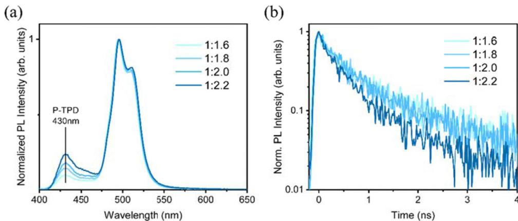
Fig. 6 (a) Normalized PL spectra and (b) time-resolved photoluminescence measurement (495 nm) of the composite film prepared by constant NPLs concentration ( $15 \text{ mg mL}^{-1}$ ) and NPLs to P-TPD ratio of 1:1.6, 1:1.8, 1:2.0, and 1:2.2.
