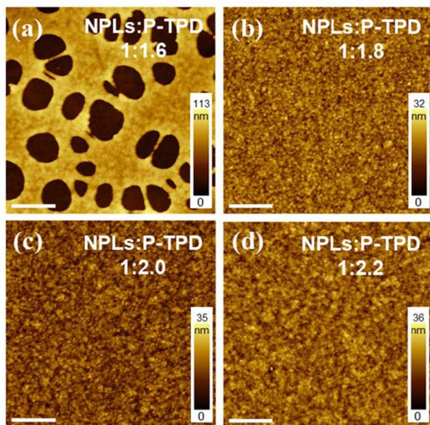
Fig. 4 AFM images showing surface morphologies of the blade-coated films using a solution with constant NPL concentration ( $15 \text{ mg mL}^{-1}$ ) and NPLs to P-TPD ratio of (a) 1:1.6, (b) 1:1.8, (c) 1:2.0 and (d) 1:2.2 with a fixed thickness of 45 nm. All white scale bars represent  $2 \mu\text{m}$ .
