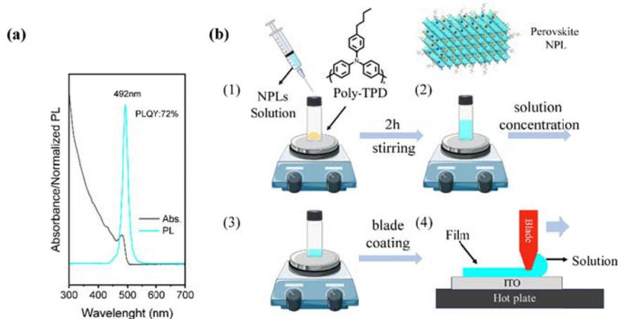
Fig. 1 (a) Absorption and PL spectra of CsPbBr<sub>3</sub> NPLs. (b) Schematic representation for polymer/NPLs composite solution preparation (ink) and the doctor-blading process for deposition.
