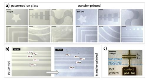
Fig. 3 (a) Selection of microscope images of the O2-patterned PEDOT:PSS thin films on glass (left) and transfer-printed on to PVA:glycerol (25 wt%) substrates (right). (b) Patterned and transfer-printed stripes (minimal width: 50 µm). (c) Patterned PEDOT:PSS on PVA:glycerol substrates with top gold contacts (thermally evaporated in vacuum) for device applications. The length of each scale bar is 500 µm.
