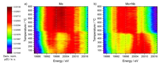
Fig. 10 Heatmap depictions of the first derivative of all recorded XANES measurements during the temperature-programmed reaction of 6Mo/HZSM-5 (a) and 6Mo1Nb/HZSM-5 (b) with 50 mL min<sup>-1</sup> 20% CH<sub>4</sub>/N<sub>2</sub> at 1 atm and a heating rate of 10 °C min<sup>-1</sup>.
