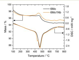
Fig. 3 Representative TG (top curves, left *y*-axis) and DSC (bottom curves, right *y*-axis) measurements over the temperature range from 100 to 800 °C on spent 6Mo/HZSM-5 and 6Mo1Nb/HZSM-5 catalysts after reaction for 360 min. Reaction conditions: 700 °C, 300 mg catalyst, 90% CH<sub>4</sub> + 10% N<sub>2</sub>, 1600 SCC  $g_{cat}^{-1}h^{-1}$ , 1 atm.
