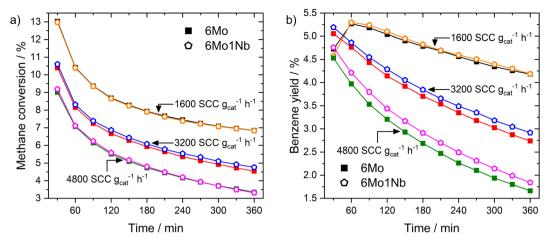
Fig. 1 Methane conversions (a) and benzene yields (b) over time for MDA reactions over 6Mo/HZSM-5 and 6Mo1Nb/HZSM-5 catalysts at different reactant flow rates. Reaction conditions: 700 °C, 300 mg catalyst, 90% CH<sub>4</sub> + 10% N<sub>2</sub>, 1 atm.
