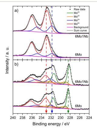
Fig. 6 Intensity-normalized XP spectra for the Mo 3d core level of fresh (a) and spent (b) 6Mo/HZSM-5 and 6Mo1Nb/HZSM-5 catalysts. Reaction conditions: 700 °C, 300 mg catalyst, 90% CH<sub>4</sub> + 10% N<sub>2</sub>, 3200 SCC  $g_{cat}^{-1} h^{-1}$ , 1 atm, 6 h. Dashed lines were added as a visual guide.
