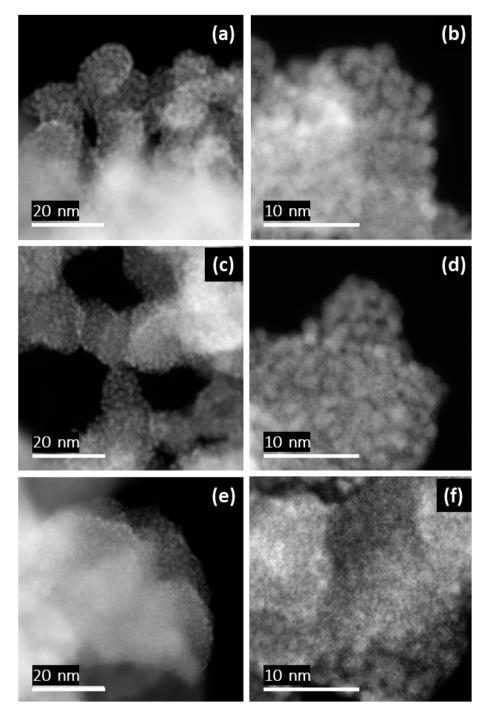
Fig. 6 HAADF STEM images of (a and b) the untreated IrO<sub>x</sub> sample, and the electrochemically treated (100 cycles, 0.0-1.65 V, 100 mV s<sup>-1</sup>) IrO<sub>x</sub> samples in (c and d) 1 M HCl and in (e and f) 1 M HCl + 20 mM CuCl<sub>2</sub> electrolytes.
