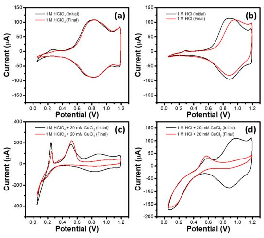
Fig. 3 CV plots of the  $IrO_x$  modified GC RDEs recorded at a scan rate of 10 mV s<sup>-1</sup> in nitrogen saturated (a) 1 M HClO<sub>4</sub>, (b) 1 M HCl (c) 1 M HClO<sub>4</sub> + 20 mM CuCl<sub>2</sub>, and (d) 1 M HCl + 20 mM CuCl<sub>2</sub> electrolytes. Labels initial and final correspond respectively to the electrodes subjected to 0 and 1600 stress cycles between 0.1 and 1.2 V at a scan rate of 1.0 V s<sup>-1</sup>.
