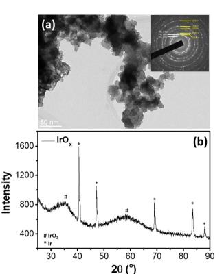
Fig. 1 (a) TEM image and (b) XRD pattern<sup>37</sup> of the studied IrO<sub>x</sub> sample.
