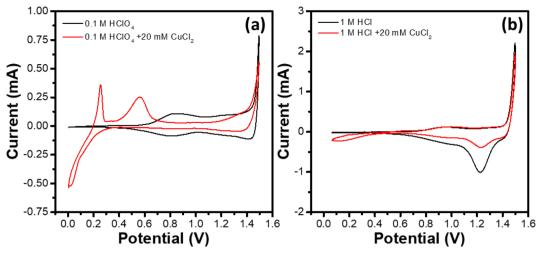
Fig. 2 Cyclic voltammograms of WE (IrO<sub>x</sub> modified GC RDE) recorded at a scan rate of 10 mV s<sup>-1</sup> in (a) 0.1 M HClO<sub>4</sub> and 0.1 M HClO<sub>4</sub> + 20 mM CuCl<sub>2</sub>, and (b) 1 M HCl and 1 M HCl + 20 mM CuCl<sub>2</sub> electrolytes saturated with nitrogen (room temperature, no rotation of WE)
