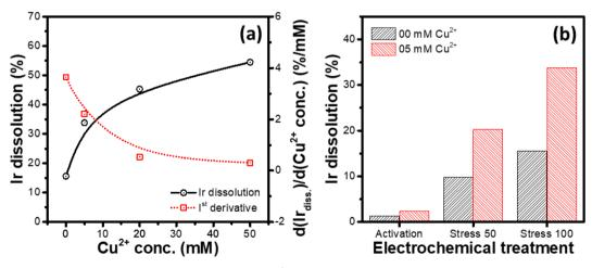
Fig. 5 (a) Variations of the Ir dissolution its first derivative with the  $Cu^{2+}$  concentration. (b) Effect of different electrochemical treatments on the Ir dissolution (activation: 100 cycles, 1 V s<sup>-1</sup>, 0-1.65 V; stress 50: activation + 50 stress cycles, 100 mV s<sup>-1</sup>, 0-1.65 V; stress 100: activation + 100 stress cycles, 100 mV s<sup>-1</sup>, 0-1.65 V) in 1 M HCl and 1 M HCl + 5 mM CuCl<sub>2</sub> electrolytes, respectively.
