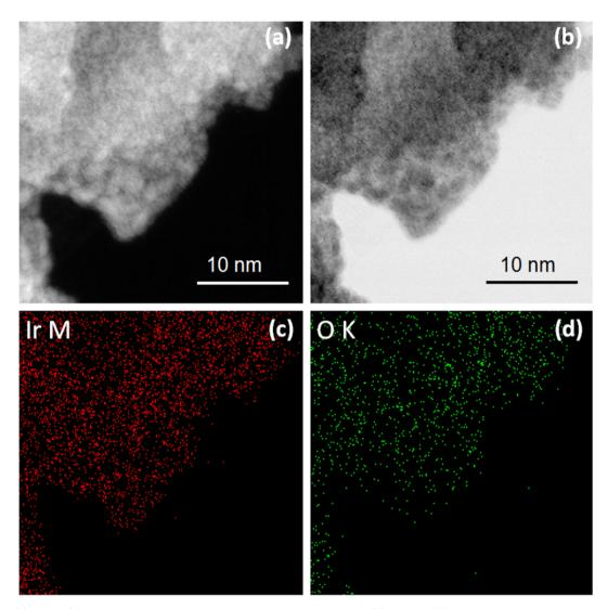
Fig. 8 HAADF (a) and BF (b) STEM images and corresponding elemental maps for Ir (c) Ir and O (d) for IrO, sample treated electrochemically in 1 M HCl + 20 mM CuCl<sub>2</sub>.
