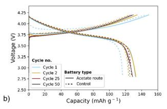
Fig. 6 Half-cell electrochemical cycling performance of NMC produced from the acetate route compared to the control NMC111 sample. (a) Discharge capacities and coulombic efficiencies of three half-cells using synthesized NMC compared to control NMC111, (b) charge-discharge profiles between 2.8 and 4.2 V for cycles 1, 2, 25, and 50 for the acetate route and the control.
