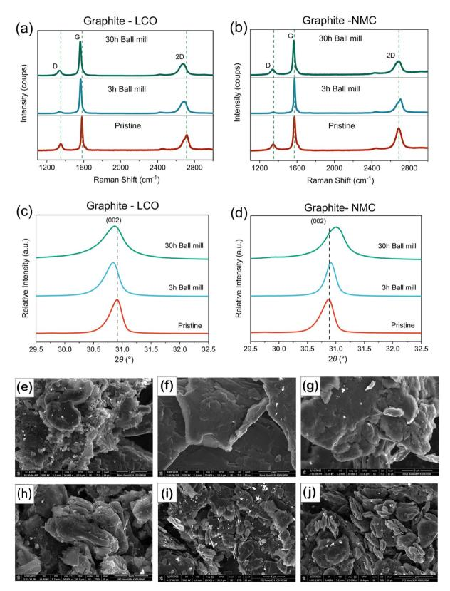
Fig. 2 Comparison of the impact of ball milling on PRG, Raman spectra of (a) PRG-LCO and (b) PRG-NMC, (c) XRD patterns in selected  $2\theta$  regions highlighting the (002) reflection of (d) PRG-LCO and (e) PRG-NMC, microstructures of (e) PRG-LCO, (f) PRG-LCO-3h, and (g) PRG-LCO-3h, and microstructures of (h) PRG-NMC, (i) PRG-NMC-3h, and (j) PRG-NMC-30h.
