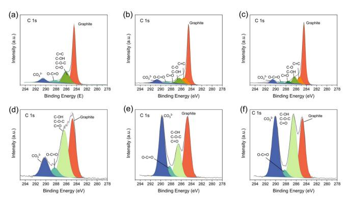
Fig. 6 C 1s XPS pattern of fresh electrodes, (a) PRG-LCO, (b) PRG-LCO-3h, and (c) PRG-LCO-30h and electrodes after 100 cycles, (d) PRG-LCO, (e) PRG-LCO-3h, and (f) PRG-LCO-30h.
