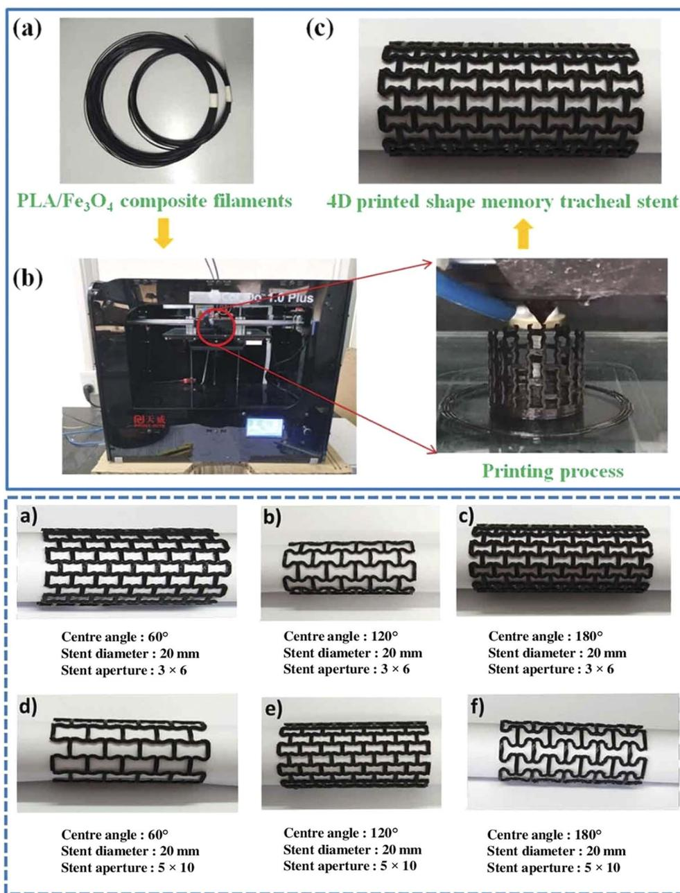
Fig. 16 (Top) (a) Filaments composed of shape memory PLA/Fe<sub>3</sub>O<sub>4</sub> composite with memory capabilities. (b) Usage of a standard FDM printer and its printing procedure. (c) Production of a tracheal stent using 4D printing technology from shape memory PLA/Fe<sub>3</sub>O<sub>4</sub> composite material. (Bottom) Tracheal stents with dynamic shape memory properties (reproduced from ref. 182 with permission from Taylor & Francis, Copyright 2021).
