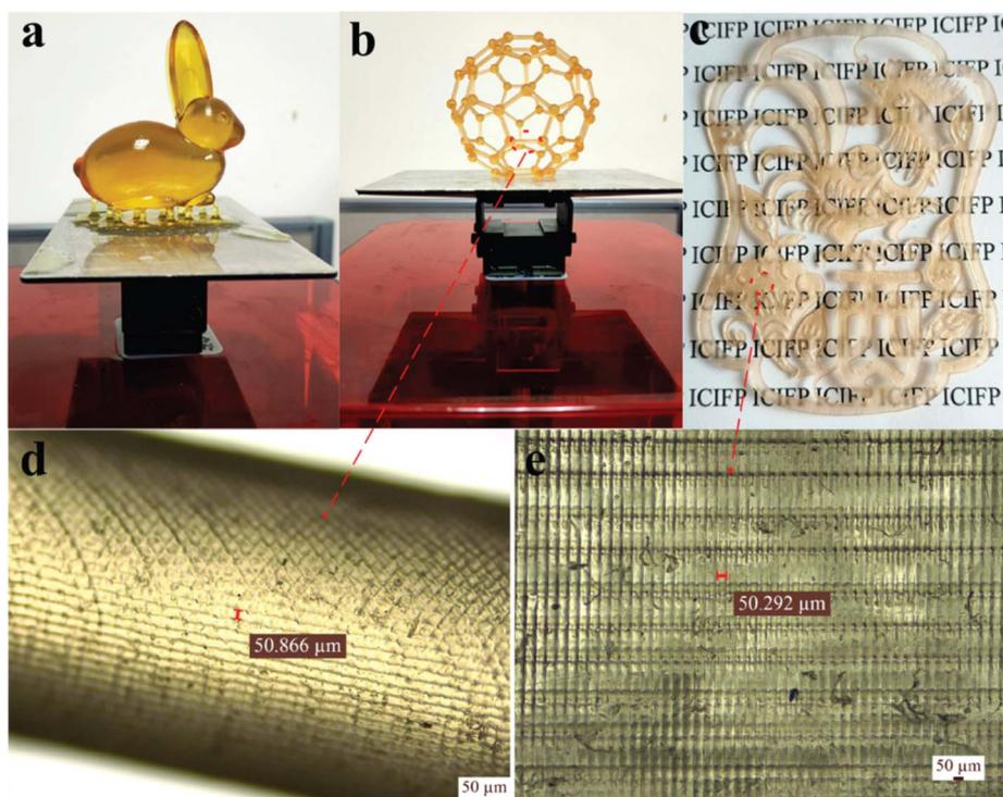
Fig. 13 Three different models produced utilizing green melanized AESO-based hybrid resin. These models include (a) rabbit model, (b) footballene model and (c) planar pattern model. Additionally, surface images of both (d) footballene model and (e) planar pattern (reproduced from ref. 145 with permission from The Royal Society of Chemistry, Copyright 2021).
