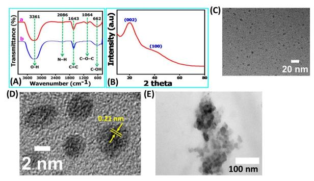
Fig. 2 Characterization and morphological analysis of NR-CDs and their interaction with Fe<sup>2+</sup> ions. (A) FT-IR spectra of neem resign extracts (dark red line) and the NR-CDs (dark blue line). (B) XRD pattern and (C and D) TEM image of the NR-CDs. (E) TEM image of NR-CDs in the presence of 62 µM of Fe<sup>2+</sup> ions.
