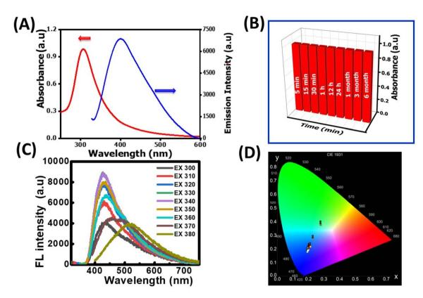
Fig. 1 Spectroscopic and photophysical properties of NR-CDs. (A) UV-vis absorption spectrum (red curve) and fluorescence spectrum (blue curve) of NR-CDs at an emission wavelength of 420 nm. (B) Time-dependent fluorescence intensity of the NR-CD probe. (C) Excitation-dependent emission spectra of NR-CDs with varying excitation wavelengths ranging from 270 to 390 nm. (D) Chromaticity coordinate diagram of NR-CDs.
