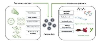
Fig. 2 Synthesis methods of CQDs and their classification.
