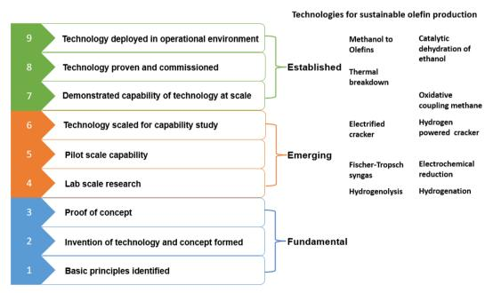
Fig. 7 Technology readiness levels (TRLs) adapted for the chemical sector with highlighted technologies for sustainable olefin production.
