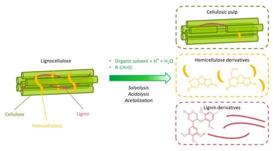
Fig. 39 Schematic outline of the AAF process for the extraction and stabilization of lignin (and hemicellulose) derivatives from lignocellulosic biomass *via* solvolysis/acidolysis and acetalization, respectively. Note: the organic solvent should be an aprotic solvent to avoid reaction of the solvent's hydroxyl groups with the aldehyde.<sup>17</sup> Moreover, the water fraction should be limited (<20% w/w) to achieve effective acetalization of lignin and carbohydrate derivates.<sup>17,18</sup>
