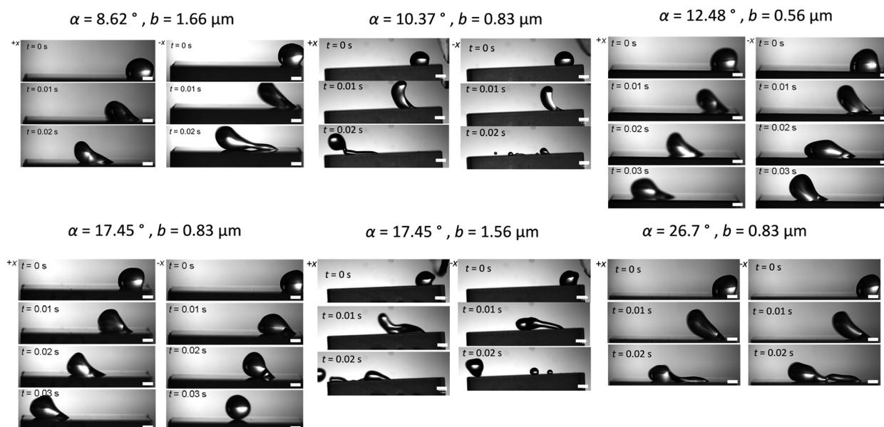
Fig. 3 Still frames of droplets being blown across glass surfaces (all scale bars 1 mm). Motion with the ridges (+x) is on the left, and against the ridges (-x) is on the right for each geometry.
