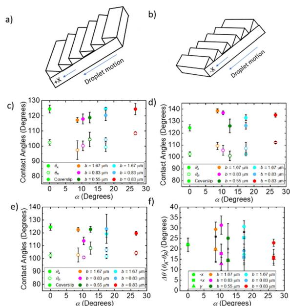
Fig. 2 (a) Schematic of the +x direction. (b) Schematic of the -x direction. (c) Droplet contact angles in +x direction vs.  $\alpha$ , surfaces imaged on a 45° tilted surface, the filled circles are advancing angles and the hollow circles are receding angles. (d) Droplet contact angles in -x direction vs.  $\alpha$ . (e) Droplet contact angles in y direction vs.  $\alpha$ . (f) Droplet contact angle hysteresis (advancing-receding).
