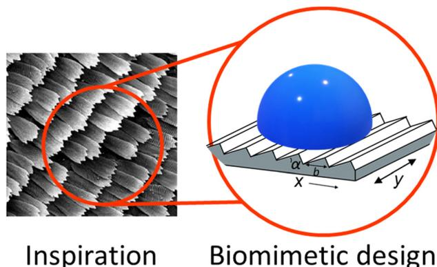
Fig. 1 Butterfly wing (shown on the left) scales served as the inspiration for our choice of surface. Blaze angle ( $\alpha$ ) blaze length ( $b$ ), the primary geometric variables are shown. The primary axes  $x$  and  $y$  are shown,  $y$  has no positive direction assigned as the surfaces are symmetric in this direction.
