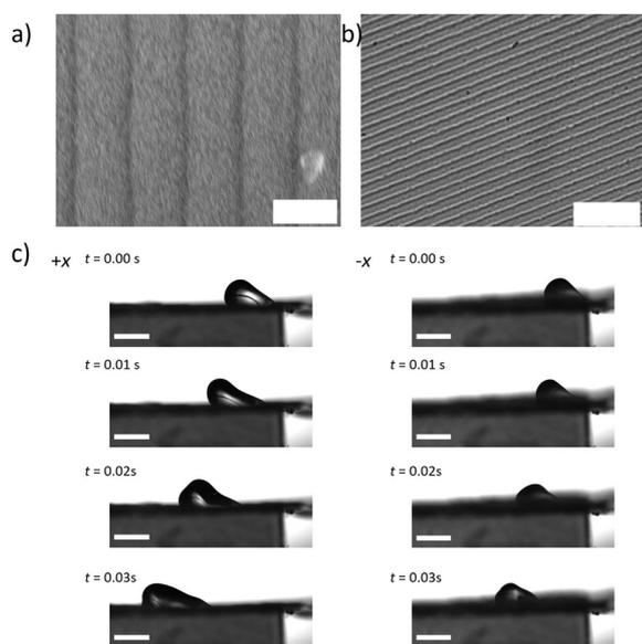
Fig. 5 (a) SEM image of PDMS imprinted surface taken at  $15\,000\times$  (scale bar is  $2 \mu\text{m}$ ). (b) Optical microscopy of imprinted surface made with Triton modified acrylate resin with  $100\times$  objective (scale bar is  $10 \mu\text{m}$ ). (c) Still frames taken showing droplet motion on Triton X-100 modified acrylate lithographs, droplet motion in  $-x$  direction is slower (scale bars are  $2 \text{ mm}$ ).
