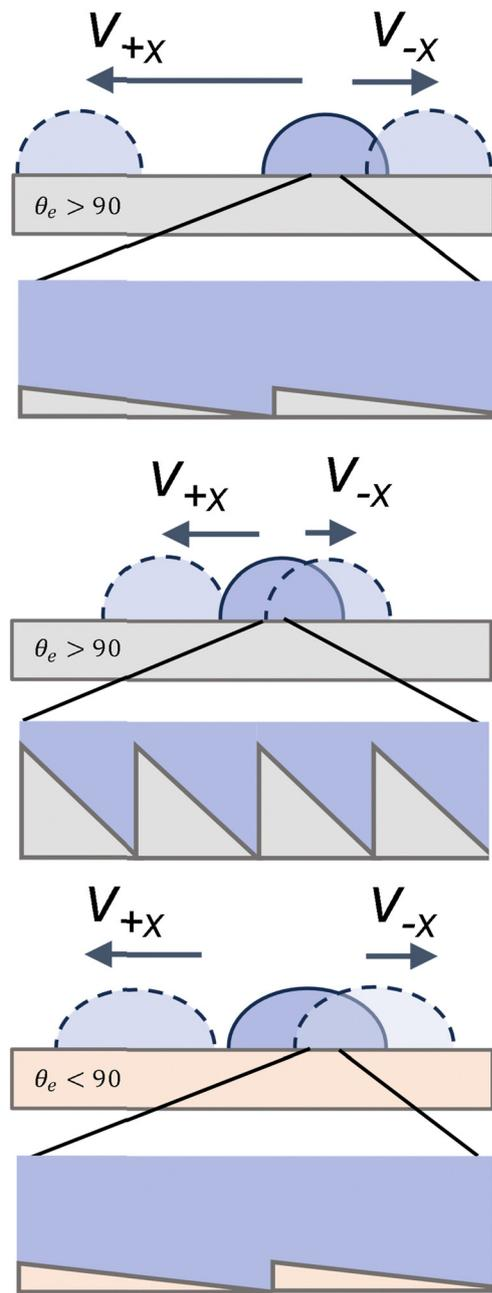
**Fig. 6** (top) Low angled surfaces have anisotropic pinning with high velocities in the  $+x$  direction and low velocity in the  $-x$  direction. (middle) High angled surfaces show strong pinning in both directions with low droplet velocities in the  $+x$  and  $-x$  directions. (bottom) Hydrophilic surfaces with anisotropic pinning with lower contact angles and velocities.
