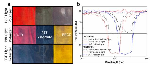
Fig. 3 (a) Visible light reflective CLC polymer coatings on PET substrates, observed through different circularly polarized light polarizers. (b) The UV-Vis-NIR transmittance spectra of the same coatings with different circularly polarized incident light.
