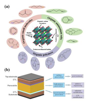
Fig. 3 (a) Depiction of the passivator molecules for different defects in WBG perovskites (b) three categories of passivation methods for WBG PVSCs.
