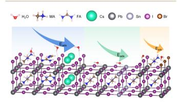
Fig. 1 Model of water adsorption on perovskite surfaces. The blue region represents water adsorption on AX-terminated surfaces, from left to right, with MA+, FA+, and Cs+ at the A-site, respectively. The green region indicates water adsorption on MX2-terminated surfaces, from left to right, with Pb2+ and Sn2+ at the M-site. The orange region represents water adsorption on MAX-terminated surfaces, from left to right, with I and Br at the X-site.
