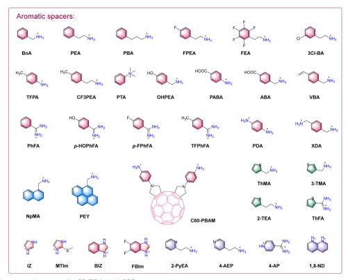
Fig. 2 Representative aromatic spacers for 2D/3D hybrid PSCs.
