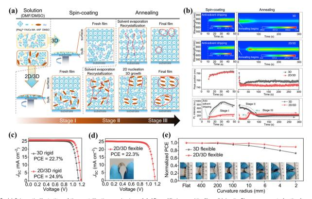
Fig. 6 (a) Schematic illustration of the crystallization mechanism of 4-AP modified perovskite films. (b) In situ PL measurements for the formation kinetics of perovskite films. J-V curves of rigid solar cells(c) and flexible solar cell (d). (e) Normalized PCE with curvature from flat to R=2 mm. Reproduced with permission.<sup>30</sup> Copyright 2023, Elsevier.
