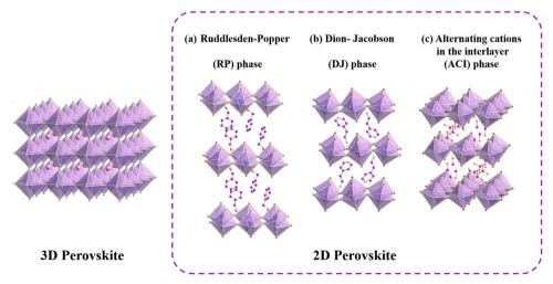
Fig. 1 Representative structures for 3D perovskite and 2D perovskite of the RP phase (a), DJ phase (b) and ACI phase (c).
