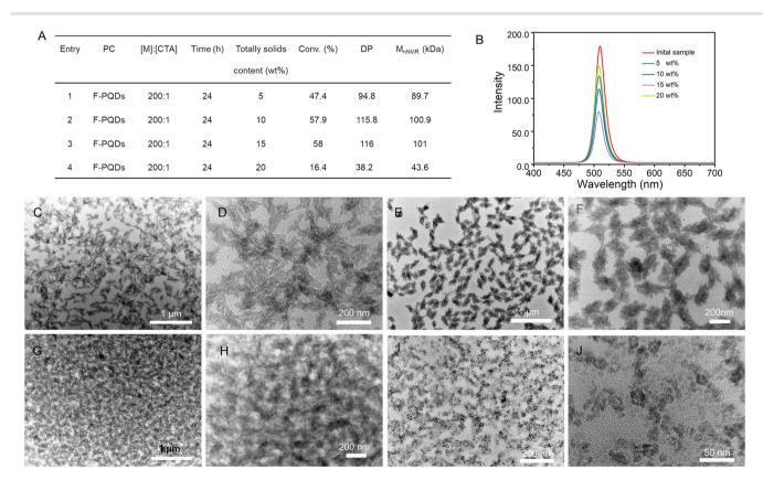
Fig. 2 (A) Characterization of POEGMA<sub>78</sub>-b-PFOEMA diblock copolymers synthesized with a different total solid content, (B) PL spectra (excited at 380 nm) of self-assembled POEGMA-b-PFOEMA nanoparticles in toluene, and (C-J) TEM images of self-assembled POEGMA<sub>78</sub>-b-PFOEMA nanoparticles.
