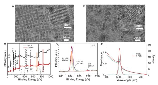
Fig. 1 (A) TEM and HRTEM images of PQDs, (B) TEM and HRTEM images of F-PQDs, (C) XPS spectra of PQDs and F-PQDs, (D) high-resolution C 1s spectra of F-PQDs, and (E) UV-vis absorption spectra and PL spectra (excited at 380 nm) of PQDs and F-PQDs in toluene.
