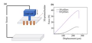
Fig. 4 A schematic of the compression force measurement and resulting force-displacement curves. (a) The compression force measurement with a maximum load cell of 50 N, (b) force vs. displacement curves for different numbers of pillars.
