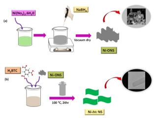
Scheme 1 (a and b) Schematic illustration of the preparation of Ni-btc  $\ensuremath{\text{NS}}$
