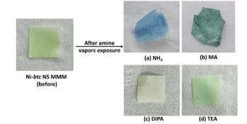
**Fig. 6** Visible color change in **Ni-btc NS MMM** upon exposure to different amine vapors.
