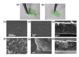
Fig. 4 (a and b) Elucidating the flexibility of membrane; (c) and (d) FESEM images of the PVDF membrane indicating smooth surface; (e) FESEM image of the cross-section of PVDF membrane; (f and g) FESEM images of Ni-btc NS MMM showing MOF NS embedded in membrane and (h) FESEM image of the cross-section of Ni-btc NS MMM.
