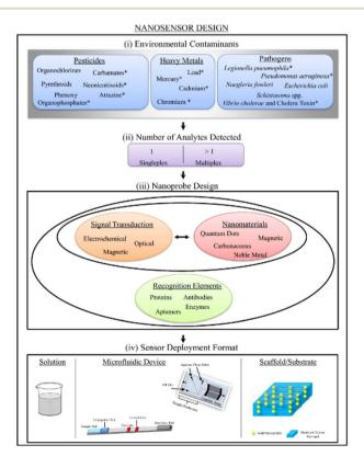
Fig. 2 Schematic representation for the design of nanosensors for environmental contaminants, also indicating the number of analytes detected, nanoprobe design, and a sensor deployment format.<sup>22</sup>
