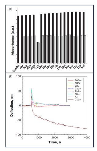
Fig. 7 (a) CuPANs' response to various amino acids; (b) bending deflection reaction to Cu<sup>2+</sup> and other cations of a silicon cantilever coated with a self-assembled monolayer of L-cysteine on the gold surface
