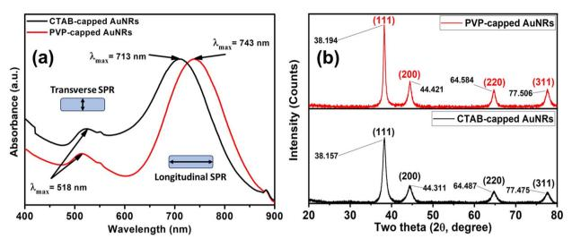
Fig. 1 (a) UV-vis absorption spectra of CTAB (black-line) and PVP capped (red-line) Au-NRs (b) XRD patterns for both CTAB-capped and PVP-capped Au NRs.
