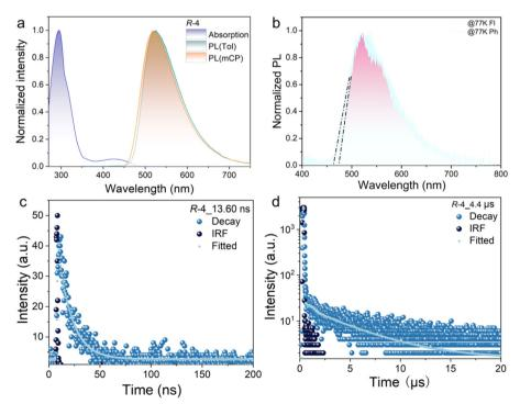
Fig. 4 (a) UV-vis spectra and PL spectra of R-4 measured in toluene solution (10<sup>-5</sup> M) and 5 wt% doped in mCP film ( $\lambda_{ex} = 420$  nm); (b) low-temperature fluorescence (FI) and phosphorescence (Ph) of R-4 doped in mCP film ( $\lambda_{ex}$  = 370 nm, delayed 2 ms); and (c) and (d) transient PL decay curves ( $\lambda_{ex}$  = 420 nm) of 5 wt% **R-4** doped in mCP film.
