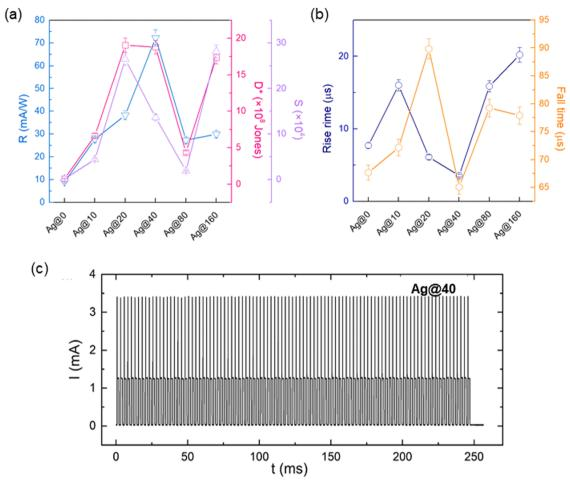
Fig. 7 (a) Responsivity (R), detectivity (D\*) and sensitivity (S) for the different samples. (b) Rise time  $(\tau_r)$  and the fall time  $(\tau_r)$  estimated for the different samples. (c) Stability of the transient response characteristics of the Aq@40 sample under zero bias and with 650 nm laser illumination and a laser power density of 887 mW cm<sup>-2</sup>.
