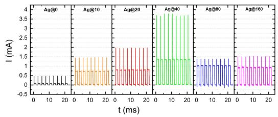
I-t curves for the different samples at a chopper frequency of 10 Hz for a fixed power density of 877 mW cm<sup>-2</sup>
