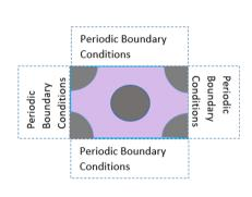
Fig. 1 (a) Computational domain used in the electromagnetic modeling. (b) Rectangular unit cell used for representing the infinite NP periodic array.
