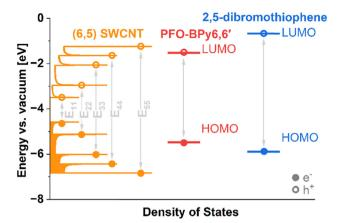
Fig. 4 Energy levels of (6,5) SWCNT, 2,5-dibromothiophene and PFO-BPy6,6', which form two type-I heterojunctions. The density of (6,5) SWCNT states (shown up to  $E_{55}$  transition) was taken from ref. 47 and aligned with the Fermi level calculated in this work ( $E_F = -4.041 \text{ eV}$ ). HOMO and LUMO levels of 2,5-dibromothiohene and PFO-BPy6,6' were also calculated in this study (cf. ESI† file).
