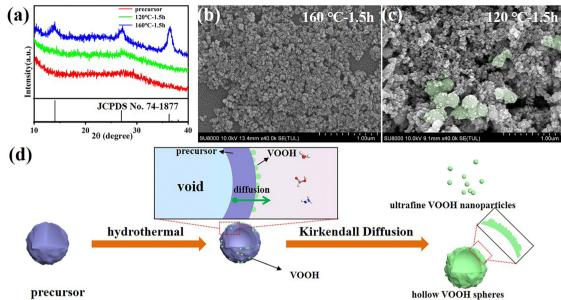
Fig. 2 (a) XRD patterns of hydrothermal precursor and hydrothermal products. SEM images of hydrothermal products under different conditions: (b) 160 °C-1.5 h and (c) 120 °C-1.5 h. (d) Schematic illustrations of Kirkendall diffusion process and the formation of ultrafine VOOH NPs.
