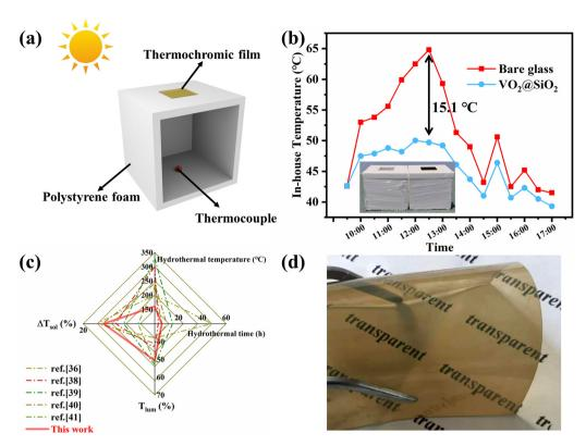
Fig. 5 (a) Schematic of the model house. (b) In-house temperature profiles of model houses (the inset shows the digital image of model houses used for the experiments). (c) Reported  $\Delta T_{sol}$  and  $T_{lum}$  of VO<sub>2</sub> obtained under different hydrothermal times and temperatures. (d) A digital image of the flexible VO<sub>2</sub> film.
