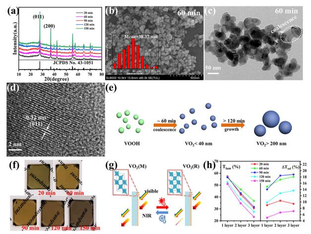
Fig. 3 (a) XRD patterns of VO<sub>2</sub> with different annealing times. (b) SEM and (c) and (d) TEM images of VO<sub>2</sub> with annealing a time of 60 min. (e) Schematic illustrations of the transformation of VOOH into VO2. (f) Digital images of VO2/PVP films. (g) Working principle of the VO2-based smart window. (h) The optical performances of VO<sub>2</sub>/PVP films with various spin coating times. (Inset (b): histogram of size distribution of the VO<sub>2</sub> NPs).
