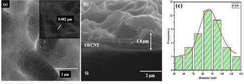
Fig. 3 SEM images of the P-SW sample: (a) top-view, (b) cross-section, and (c) diameter distribution curve
