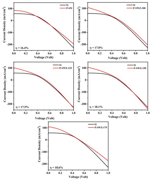
Fig. 12 J-V curve of SWCNT and SWCNT/ZnO NCs integrated Si thin film
