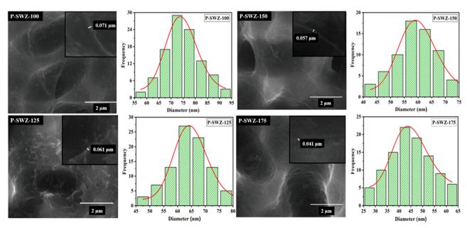
Fig. 4 SEM images of SWCNT/ZnO NC integrated Si thin films prepared at various annealing temperatures.
