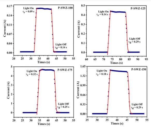
Fig. 10 Photoresponse current fitting of SWCNT/ZnO NCs on Si thin films.
