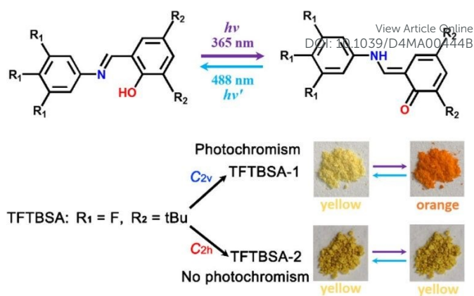
Figure 10: Conversion of enol form to trans -keto form and vice versa upon UV light irradiation (up) and photochromic and non-photochromic behaviour of the polymorphic forms TFTBSA-1 and TFTBSA-2, respectively. tBu = tert -butyl. Reprinted (used in part) with permission from reference 75 . Copyright 2021 American Chemical Society.
