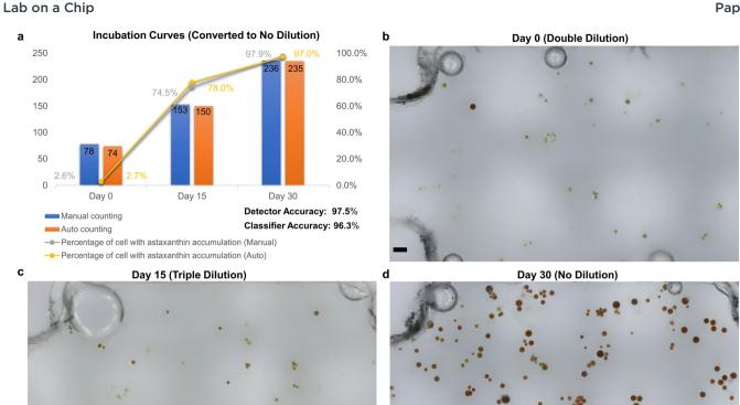
Fig. 5 Monitoring the accumulation of astaxanthin in Haematococcus Pluvialis. a) Culture experiment data and comparison graph of manual and AIMP obtained statistics. Example images of a single observation chamber at b) day 0 (samples are diluted twofold before adding to the chip), c) day 15 (samples are tripled diluted before adding to the chip), and d) day 30 (samples are not diluted). Scale bars are 200 µm.
