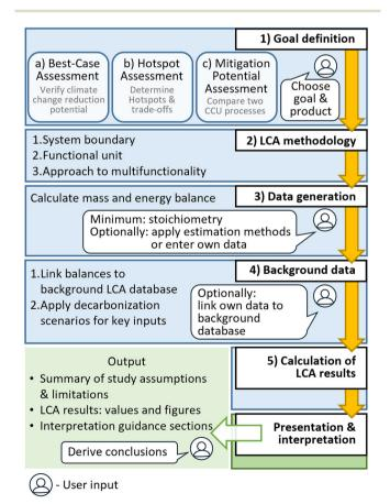
Fig. 1 Overview of the ESTIMATe method and user inputs in each step. CCU – carbon capture and utilization.
