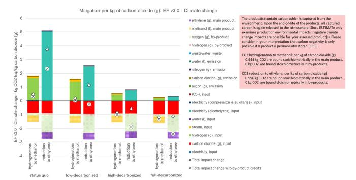
Fig. 8 Climate Change Impact results of the Mitigation Potential Assessment comparing electrochemical  $CO_2$  reduction to ethylene (left bars) and  $CO_2$  hydrogenation to methanol (right bars) in the ESTIMATe tool. The different bar clusters correspond to the different background system scenarios defined in section 2.4.
