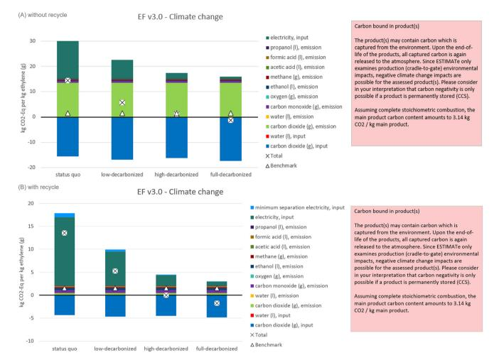
Fig. 5 Climate Change Impact of laboratory-scale electrochemical CO2 reduction to ethylene in the ESTIMATe tool. (A) Without recycle of unreacted CO2, (B) including a recycle of unreacted CO2. Note the different scales of the y-axes. The different bars correspond to the different background system scenarios defined in section 2.4.
