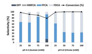
Fig. 4 Effect of buffer (acetate pH 4.5 and citrate pH 6.0) and ionic strength (25, 50, 75, and 100 mM, respectively) in the selectivity and conversion on the oxidation HMF by LacTV-TEMPO system. Reaction condition: HMF (25 mM), TEMPO (0.3 equivalents), LacTV (5 U), reaction time (48 h), 30 °C and 300 rpm.
