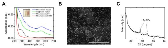
Fig. 3 Au nanoparticle (NP) formation in the mixed-metal solution. (A) UV-vis absorption of Au nanoparticles in the mixed-metal solution both with and without the presence of mucin. Inset: Optical image of mixed-metal solution before (left) and after (right) the addition of mucin. (B) Scanning electron microscope (SEM) image of Au nanoparticles formed in the mixed-metal solution in the presence of mucin. (C) X-ray diffraction (XRD) pattern of the mixed-metal precipitate after centrifugation.
