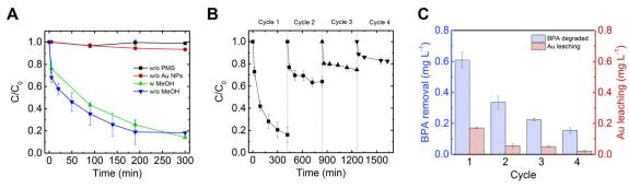
Fig. 5 Peroxymonosulfate (PMS) activation for bisphenol A (BPA) degradation. (A) Removal of BPA with PMS and Au nanoparticles in dispersion.  $[BPA]_0 = 1 \text{ mg L}^{-1}$ ;  $[PMS]_0 = 0.2 \text{ mM}$ ;  $[Au NPs]_0 = 0.015 \text{ g L}^{-1}$ . (B) Removal of BPA with Au nanoparticle-embedded mucin nanofibers (in the presence of PMS) over four cycles. (C) BPA removal by Au-embedded nanofibers (blue) and Au leaching (red) for each cycle in (B).
