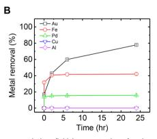
Fig. 1 (A) Metal removal by mucin from mixed-metal and isolated-metal aqueous solutions (initial concentration of each metal: 0.05 mM in steady state). (B) Removal of all metals by mucin as a function of time from an aqueous mixed-metal solution containing 0.05 mM of each metal. All experiments were conducted in  $0.1 \text{ g L}^{-1}$  dissolved mucin and solution pH of 4. Error bars represent one standard deviation from an average of two measurements.
