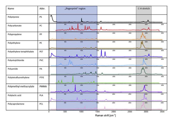
Fig. 10 RSA of polymers' fingerprint region and region for C-H stretching modes of alkyls, alkenes, and aromatic protons (License: Under Creative Commons CC-BY).<sup>56</sup>
