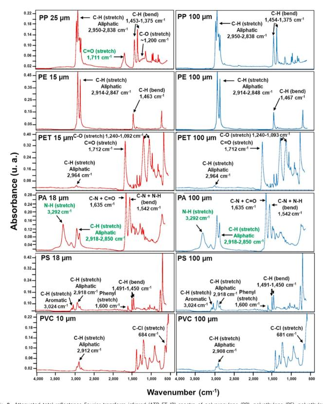
Fig. 9 Attenuated total reflectance Fourier transform infrared (ATR FT-IR) spectra of polypropylene (PP), polyethylene (PE), polyethylene terephthalate (PET), polyamide (PA), polystyrene (PS), and polyvinyl chloride (PVC) (License: Under Creative Commons CC-BY).51
