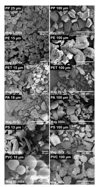
Fig. 12 SEM images of PP, PE, PET, PA, PS, and PVC with the magnification of the images ranging from  $297 \times$  to  $50\,000 \times$  (License: Under Creative Commons CC-BY).<sup>51</sup>
