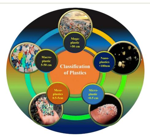
Fig. 2 Classification of different types of plastics discovered in the surrounding environment (License: Under Creative Commons 3.0).
