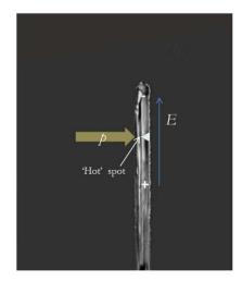
Fig. 4 Schematic presentation of the cracking of a growing column ice crystal (growth + cracking) under the influence of pressure (p). The blue arrow represents an electric field E. The 'Hot' spot is a point at the tip of a crack with a highly localized electric field  $E^{Cr}_{\perp}$ .
