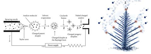
Scheme of electrospray ionization in a mass-spectrometer
