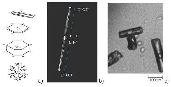
Fig. 3 (a) Charge distribution in growing ice crystals of various habits generating electric 'multipoles' (reproduced from ref. 61 with permission from Elsevier, copyright 1988); (b) distribution of charge during ice growth – H<sup>+</sup> and L<sup>-</sup> defects are concentrated inside the crystal, OH- and Ddefects on the tips; (c) T-shape ice crystal aggregates as a result of charging (reproduced from ref. 61 with permission from Elsevier, copyright 1988).
