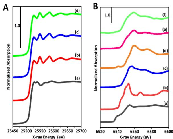
**Fig. 6** [A] Ag K-edge XANES of (a) Ag<sub>2</sub>O, (b) Ag foil, (c) the Ag(1)/BT4 sample, and (d) the Ag(1)-MnO<sub>x</sub>(0.492)/BT4 sample. [B] Mn K-edge XANES of (a) Mn foil, (b) MnO, (c) Mn<sub>2</sub>O<sub>3</sub>, (d) MnO<sub>2</sub>, (e) the MnO<sub>x</sub>(0.580)/BT4 sample, and (f) the Ag(1)-MnO<sub>x</sub>(0.492)/BT4 sample. The BT4 sample used was the BT4(20,1273) sample.
