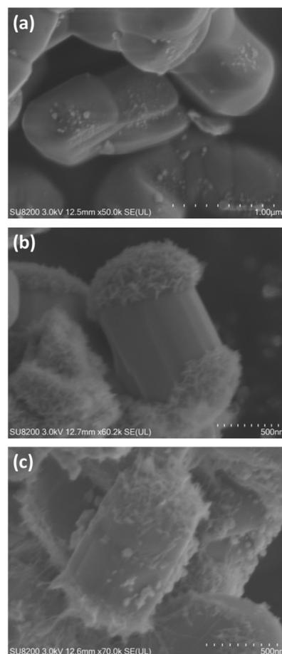
**Fig. 7** SEM images of the samples: (a) Ag(1)/BT4, (b) MnO<sub>x</sub>(2.4)/BT4, and (c) Ag(1.499)-MnO<sub>x</sub>(0.523)/BT4. The BT4 sample used was BT4(20,1273).
