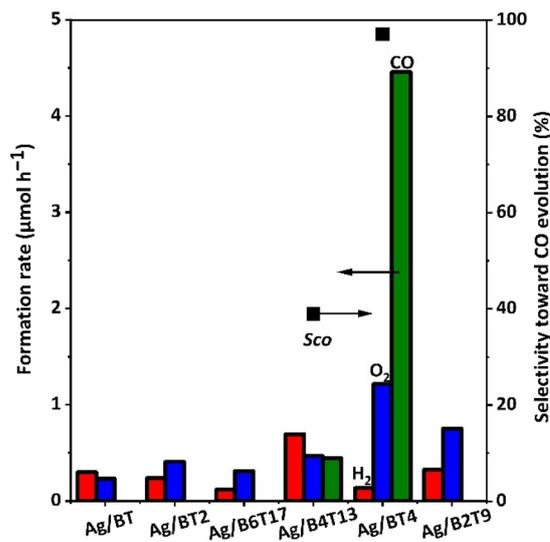
Fig. 2 Formation rates of H<sub>2</sub> (red), O<sub>2</sub> (blue), and CO (green), and selectivity for CO evolution ( $S_{CO}$ , square) in the photocatalytic reaction test for CO<sub>2</sub> reduction with water under photoirradiation over the barium titanate samples with 1 wt% Ag cocatalyst.
