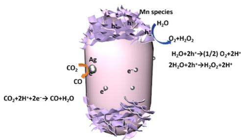
Fig. 8 Schematic drawing of photocatalytic CO<sub>2</sub> reduction with water as an electron donor on the Ag-MnO<sub>x</sub>/BT4 crystal photocatalyst.
