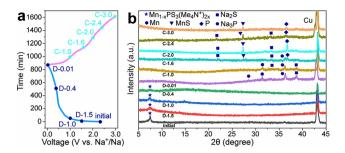
Fig. 5 (a) Initial charge-discharge curve of the  $Mn_{1-x}PS_3(Me_4N^+)_{2x}$ electrode at 0.05 A g<sup>-1</sup> and (b) corresponding ex situ XRD patterns at different voltage stages. Reproduced with permission from ref. 132. Copyright (2024), Elsevier.
