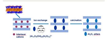
Fig. 1 Preparation of Al<sub>2</sub>O<sub>3</sub> pillared clays.
