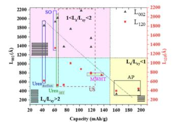
Fig. 9 Correlation between the capacities obtained from the CV of the first cycle and structural coherence lengths  $L_z$  and  $L_{xY}$  obtained from the XRD analysis for the Cu<sub>2</sub>(OH)<sub>3</sub>(NO<sub>3</sub>) series of samples with US: ultrasonification, AP: alkaline precipitation, MWHT: microwave high-temperature, and SO: salt and oxide method. Reproduced with permission from ref. 185. Copyright (2023), the American Chemical Society.
