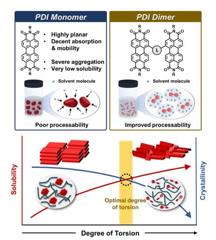
Fig. 4 General design rules for achieving PDI dimers and multimers with balanced solubilities and aggregation properties through tuning molecular planarity.
