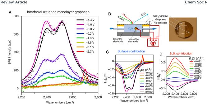
Fig. 10 (A) In situ SFG spectra of D<sub>2</sub>O at the graphene electrode (no electrolyte is added to D<sub>2</sub>O). The potential is referenced to a Ag/AgCl electrode. (B) Schematic of an electrochemical cell and the corresponding photograph of a graphene electrode for SFG experiments. (C) and (D) The extracted surface (C) and bulk (D) contribution from SFG spectra as a function of the applied field. Reproduced with permission from ref. 140. Copyright 2021 Springer Nature
