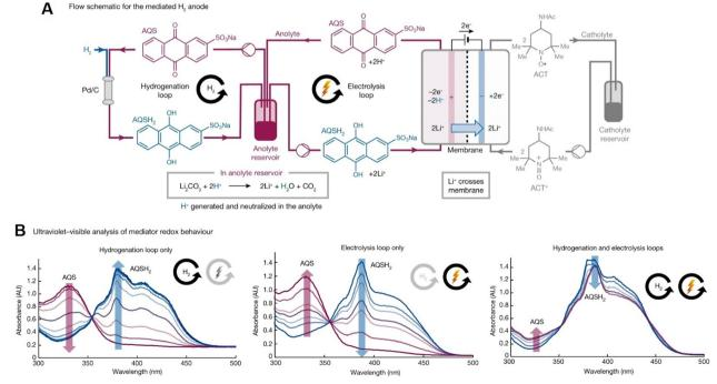
Fig. 18 (A) Schematic of mediated H<sub>2</sub> anode by paring the thermal hydrogenation of AQS and the electrochemical oxidation of AQSH<sub>2</sub> in real time. (B) In situ UV-Vis spectra of the redox speciation of AQS and AQSH<sub>2</sub> species in the analyte reservoir for various processes, such as hydrogenation-only or electrolysis-only loop, or both loops operating simultaneously. Reproduced with permission from ref. 215. Copyright 2023 Springer Nature
