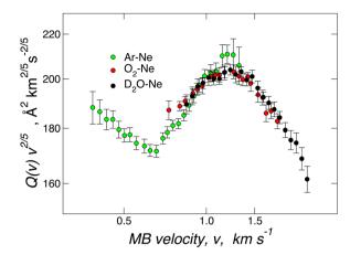
Fig. 2 Total integral cross-sections Q(v) for collisions between Ar (green),  $O_2$  (red) and  $O_2O$  (black) and Ne measured at selected beam velocity v. As usual,  $^{41-43,58}$  data are plotted as  $Q(v) \cdot v^{2/5}$  to emphasize the glory patterns. Reproduced from ref. 25 with permission from American Chemical Society, copyright © 2012.
