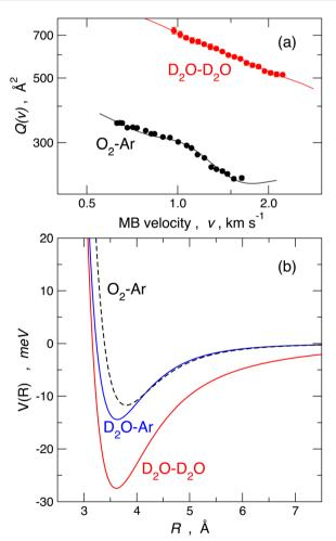
Fig. 6 Panel (a): comparison of the measured Q(v) data. Panel (b): the best fit experimental interaction potential for  $O_2$ –Ar (black dashed, van der Waals),  $D_2O$ –Ar (blue continuous, weak HB) and  $D_2O$ – $D_2O$  (red, strong HB): 1 meV = 0.096485 kJ mol<sup>-1</sup>. Spherically averaged potentials are plotted and used for the scattering cross-section calculation reported in panel (a).
