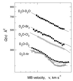
Fig. 13 Comparison of the integral cross-sections Q(v) measured, under the same experimental conditions, for the scattering of D<sub>2</sub>O molecular beams, velocity selected in the v range, by Br2, Cl2 and other selected targets.
