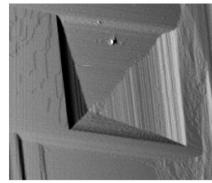
Fig. 14 Left: An illustration of step edges, kinks and etch pits. Reproduced with permission from Arvidson et al., Geochim. Comochim. Acta. 2003, 67, 1623. Copyright 2003 Elsevier. 95 Right: An AFM image of an etch pit reproduced with permission from Shiraki et al., Aquat. Geochem., 2000, 6, 87. Copyright 2000 Kluwer Academic Publisher. 96 The etch pit is about 3 µm wide
