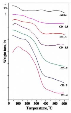
**Fig. 16** TGA curves for calcite modified by stearic acid. The data is shown for calcite powder and samples with different degree of coverage given within brackets. CD-0.5 (0.52), CD-1 (1.00), CD-1.5 (1.53), CD-2 (2.16), CD-3 (3.25), CD-4 (4.44). Figure reproduced with permission from Mihajlovic *et al.*, *Powder Technol.*, 2013, **245**, 208. Copyright 2013 Elsevier.<sup>123</sup>
