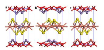
Fig. 8 Crystal structure of (a)  $C_1M_3OS$ , (b)  $C_1M_1OS$ , and (c)  $C_3M_1OS$ , where orange, purple, yellow, and red are Cu, Mn, S, and O atoms, respectively.
