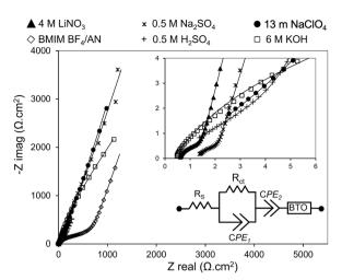
Fig. 8 EIS measurements of coal char electrodes presented as a normalized Nyquist plot. Upper inset: High-frequency behavior. Lower inset: Randles equivalent circuit model with series resistance  $R_{s_r}$  charge transfer resistance  $R_{ct}$ , constant phase elements (CPE<sub>1</sub> and CPE<sub>2</sub>), and Bisquert Open (BTO) circuit elements
