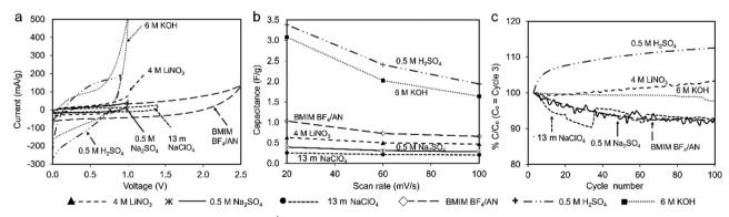
Fig. 5 (a) CV curves for all tested electrolytes (100 mV s<sup>-1</sup>). (b) Specific capacitance at different scan rates for each electrolyte. (c) Capacitance retention (% of cycle 3 specific capacitance) over 100 cycles (100 mV s<sup>-1</sup>).
