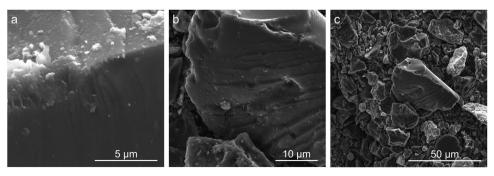
Fig. 1 SEM images of Sufco coal char particles post-pyrolysis.
