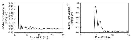
Fig. 2 Pore size distribution of coal char post-pyrolysis calculated from (a) N<sub>2</sub> and (b) CO<sub>2</sub> adsorption measurements.
