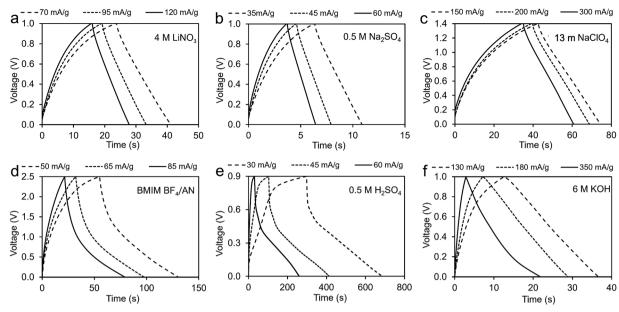
Fig. 7 GCD measurements of coal char in: (a) 4M LiNO<sub>3</sub>, (b) 0.5 M Na<sub>2</sub>SO<sub>4</sub>, (c) 13 m NaClO<sub>4</sub>, (d) BMIM BF<sub>4</sub>/AN, (e) 0.5 M H<sub>2</sub>SO<sub>4</sub>, and (f) 6 M KOH electrolytes.
