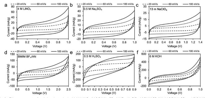
Fig. 4 CV measurements of coal char electrodes in: (a) 4 M LiNO<sub>3</sub>, (b) 0.5 M Na<sub>2</sub>SO<sub>4</sub>, (c) 13 m NaClO<sub>4</sub>, (d) BMIM BF<sub>4</sub>/AN, (e) 0.5 M H<sub>2</sub>SO<sub>4</sub> and (f) 6 M KOH at scan rates of 20, 60, and 100 mV  $s^{-1}$ .
