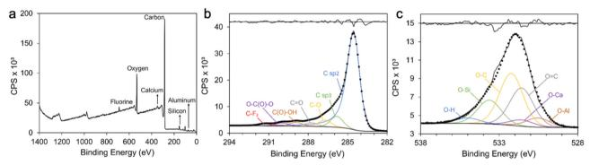
Fig. 3 XPS spectra of coal char including: (a) survey spectra; (b) C1s and (c) O1s narrow scans. Residual standard deviations of peak fittings are provided in (b) and (c) (upper black lines).
