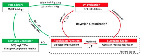
Fig. 5 A schematic representation of BO guided computational workflow for identify HBEs with desired oxidation potentials. PCs,  $\mu$  and  $\Sigma$  are principle components, mean, and variance, respectively. Reproduced with permission from ref. 93. Copyright American Chemical Society 2020
