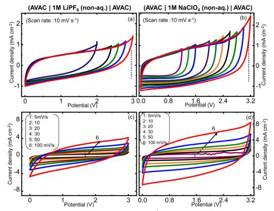
Fig. 8 (a and b) CV curves at different potential windows at a scan rate of 10 mV s<sup>-1</sup> and (c and d) cyclic voltammograms at different scan rates for the dual carbon lithium-ion capacitor (left) and dual carbon sodium-ion capacitor (right) devices in the CR-2032 coin cell.
