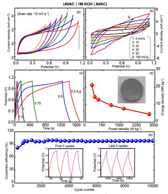
Fig. 7 (a) CV profiles recorded at different potential windows at a scan rate of 10 mV s<sup>-1</sup>, (b) cyclic voltammograms at different scan rates, (c) GCD curves at different current densities, (d) Ragone plot, and (e) cycle-life data at 2 A g<sup>-1</sup> recorded for the aqueous supercapacitor (AVAC|1 M KOH|AVAC) in the CR-2032 coin cell. Inset: Charge-discharge profiles of the first three and last three cycles.
