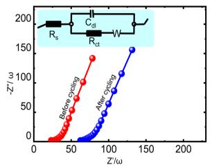
Fig. 10 Nyquist plots recorded for the dual carbon sodium-ion capacitor before, and after cycle life. Inset: Equivalent circuit used for fitting the Nyquist plot.
