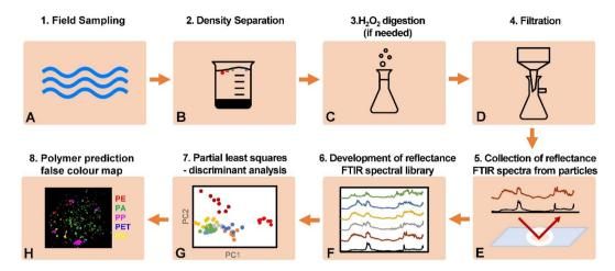
Fig. 1 Flow diagram of the protocol for reflectance-FTIR detection of microplastics in environmental samples.
