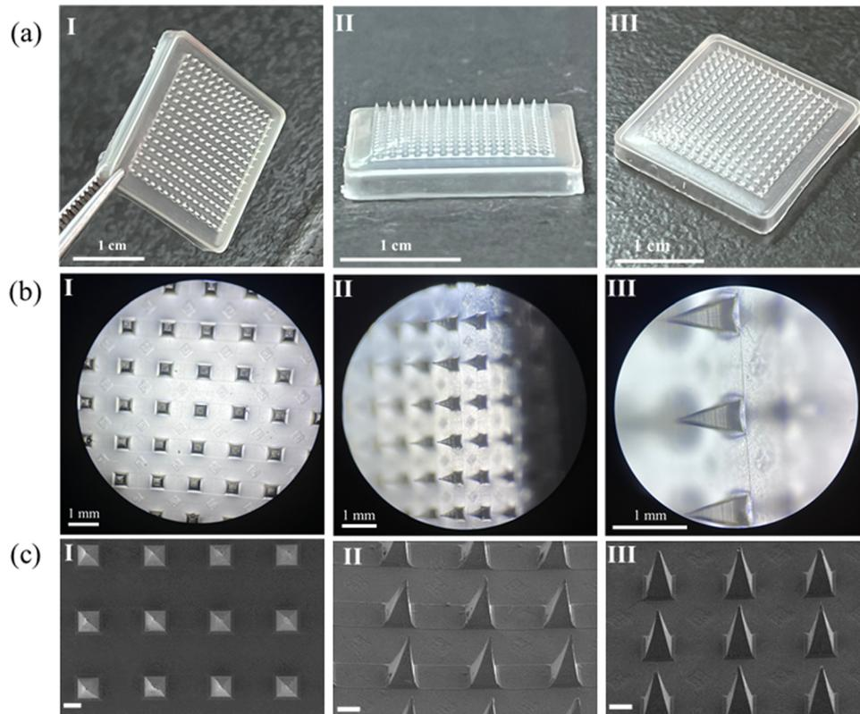
Fig. 3 Morphological characterization images of dissolving HA MNs containing CS-MoS<sub>2</sub>. The direct view of the MNs taken using a mobile phone (a); the shape of the MN tips under an optical microscope (b); the SEM images of the dissolving HA MNs containing CS-MoS<sub>2</sub> (c), scale bars: 200 μm.
