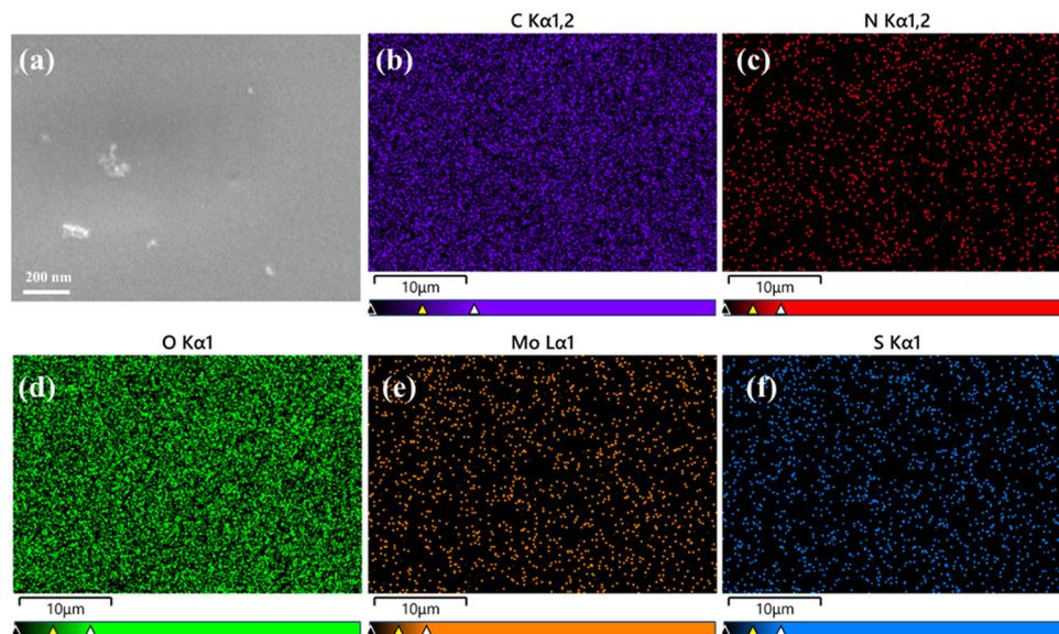
Fig. 4 SEM image of dissolving HA MNs containing CS-MoS<sub>2</sub> (a) and the corresponding elemental mapping for C (b), N (c), O (d), Mo (e), and S (f) dissolving HA MNs containing CS-MoS<sub>2</sub>.
