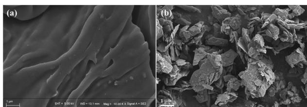
Fig. 2 SEM images of the prepared CS-MoS<sub>2</sub> (a) and the original MoS<sub>2</sub> (b).
