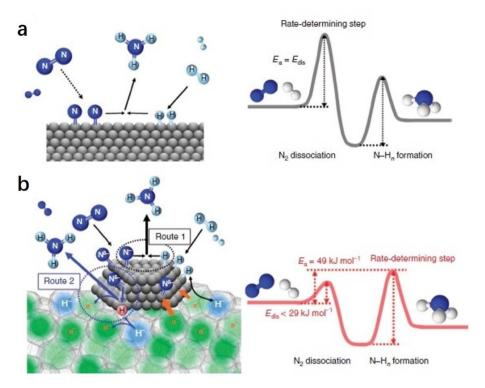
Fig. 7 Reaction mechanism and energy diagram for NH<sub>3</sub> synthesis on (a) conventional catalyst and (b) Ru/C12A7:e<sup>-</sup> catalyst. Copyright 2015, Springer Nature.
