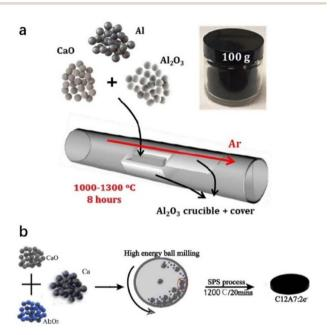
Fig. 3 (a) Schematic of aluminothermic synthesis of C12A7:e<sup>-</sup> *via* one-step calcination of mixtures of oxide and Al. Inset is an image of 100 g mass-produced C12A7:e<sup>-</sup> powders. Copyright 2019, American Chemical Society. (b) Schematic of the synthesis process of C12A7:e<sup>-</sup> *via* SPS of mixtures of oxide and Ca. Copyright 2019, Elsevier.
