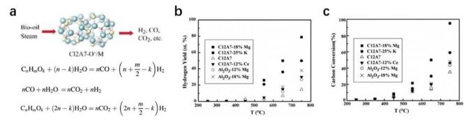
Fig. 19 (a) Steam reforming of biomass. The hydrogen yield (b) and (c) carbon conversion from the catalytic steam reforming of the bio-oil were measured as a function of temperature over various catalysts. Copyright 2007, Elsevier.
