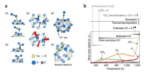
Fig. 15 (a) Geometrical configurations of a CO<sub>2</sub> molecule adsorbed on C12A7:e<sup>-</sup> surface. (b) TPD curves of all desorption products from the C12A7:e surface after 2 L of exposure to CO2 at RT with the proposed CO2 desorption and decomposition sequence. The intensities of the curves were calibrated using sensitivity factors. Copyright 2013, Springer Nature.
