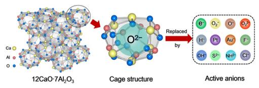
Scheme 1 Structures of C12A7 and single cage structure and exchangeable active anions.
