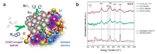
Fig. 24 (a) Schematic diagram of the ammonia synthesis reaction over Ru/C12A7:e<sup>-</sup>. (b) The inelastic neutron-scattering spectra of Ru/C12A7:e<sup>-</sup> collected at 5 K after exposure to (1) 0.1 MPa 3:1 H<sub>2</sub>: N<sub>2</sub> mixture, (2) vacuum, (3) 0.1 MPa H<sub>2</sub>, and (4) 5 cycles of 0.1 MPa N<sub>2</sub> at 673 K. Copyright 2020, American Chemical Society,
