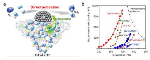
Fig. 8 (a) Reaction mechanism for NH<sub>3</sub> synthesis on Co/C12A7:e<sup>-</sup> catalyst. (b) Temperature dependence of NH<sub>3</sub> synthesis rate for the supported Co catalysts. Reaction conditions: WHSV, 18 000 mL  $g^{-1}$   $h^{-1}$ ; pressure, 0.1 MPa. Copyright 2019, American Chemical Society.
